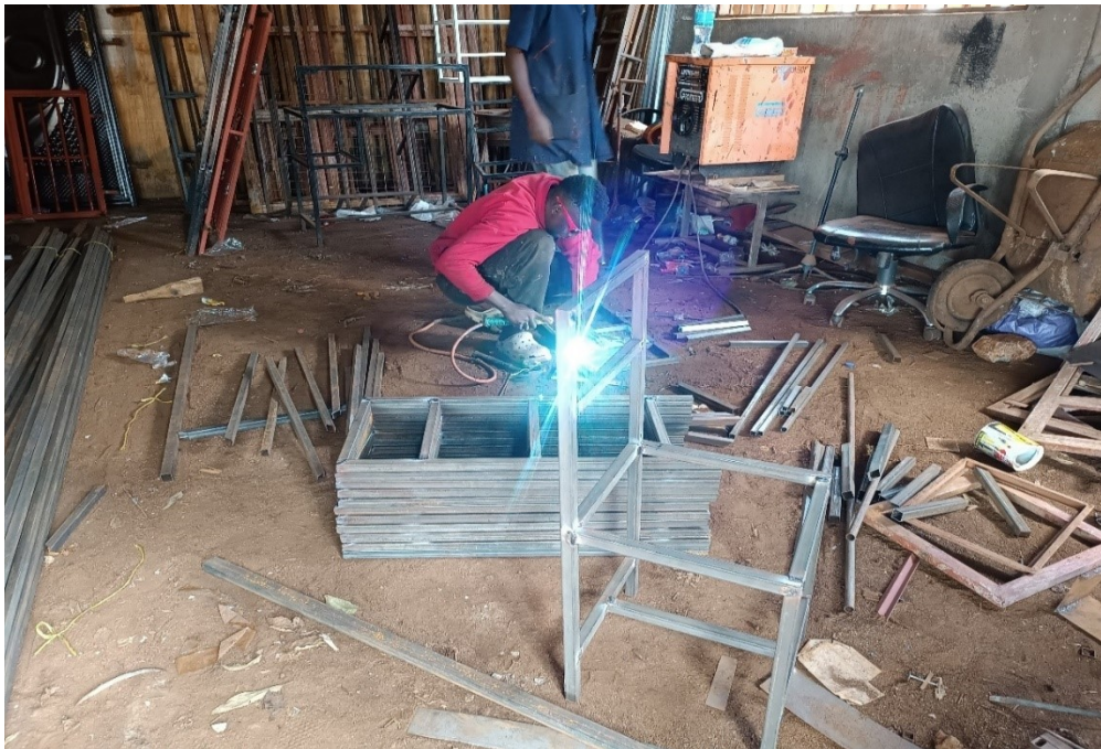
The second stage was to prepare the steel for connecting with wood to make desks, chairs and tables. As the photo shows welder welding steel to make desks.
